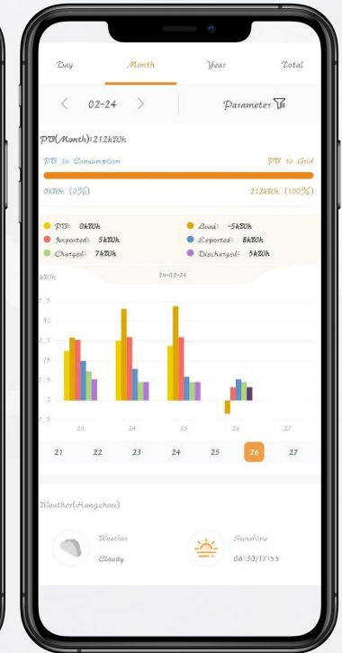
Real time recording of power generation, storage, and consumption
