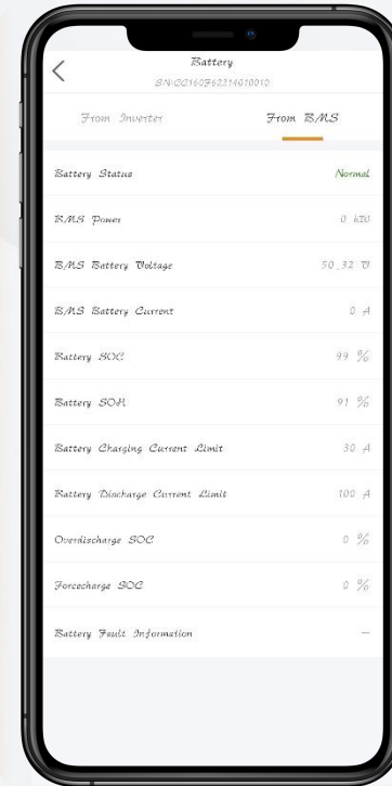
Real time monitoring of battery status
